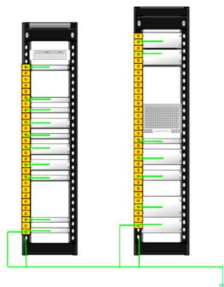
Figura 38: Connecting the Racks to the Ground Wire Source: [13]
