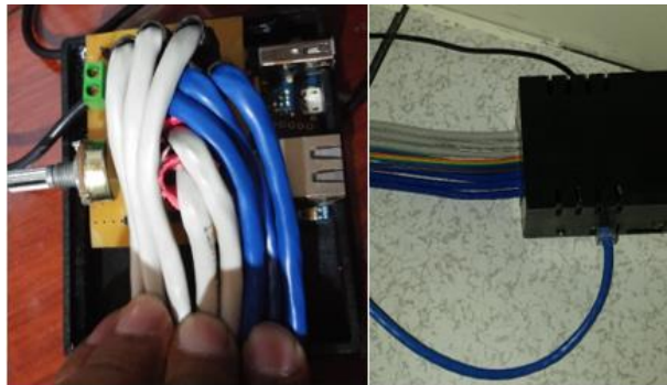
Figure 15 Placement of the Arduino in the box.
