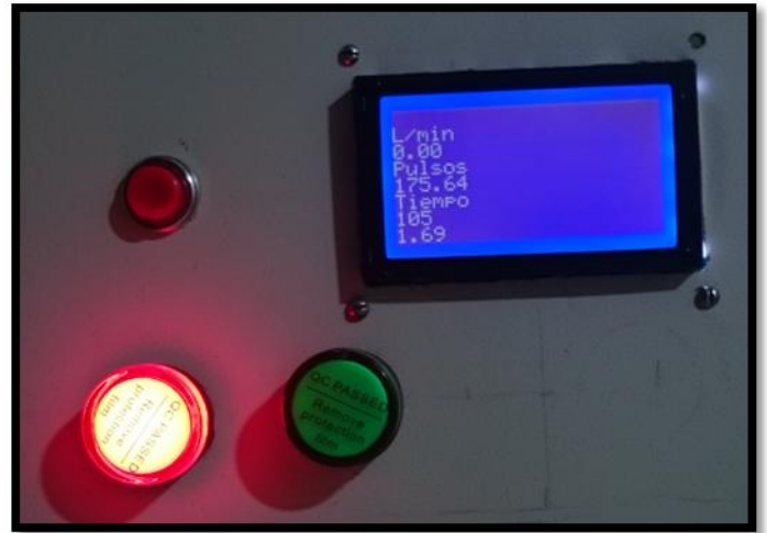
Figure 28 On pilot light to indicate end of milk extraction process
