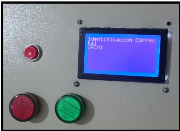
Figure 22 Message of "Correct identification" of the bovine in GLCD
