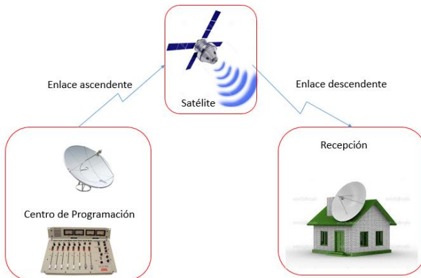
Fig. 3: Satellite Broadcasting scheme
