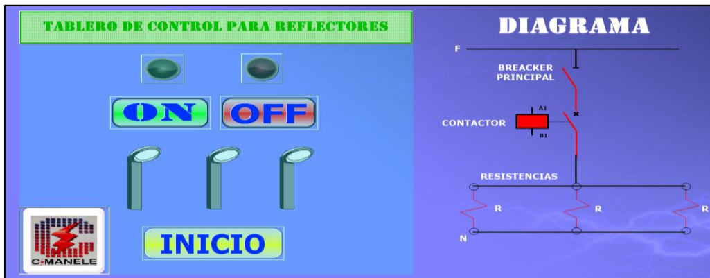
Figura 82: Control de reflectores (MOVICON 11.5)
