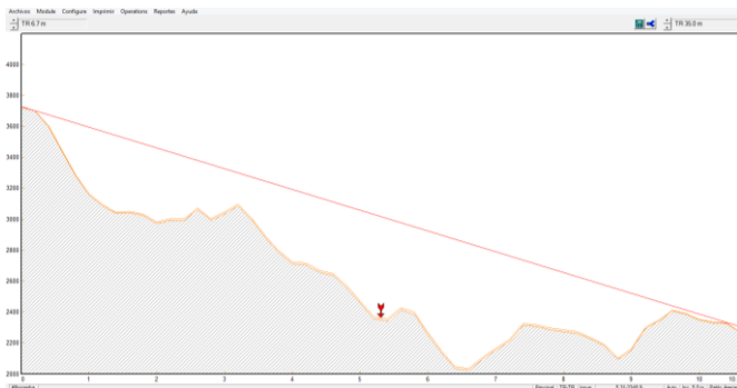
Figure 6: Example of profile of terrain elaborated in the software PathLoss
