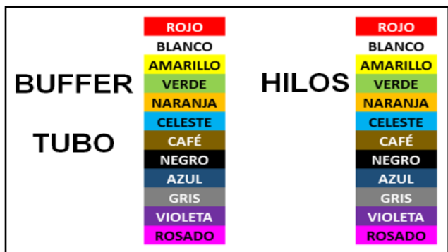
Figure # 7. Color buffers and threads of 144 threads fiber-optic cable.
