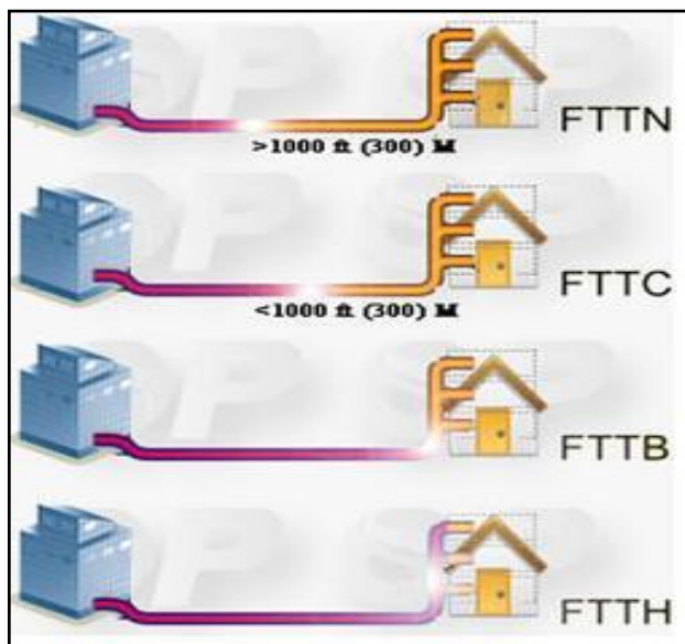
Figure # 3. Optical fiber to the home.
