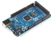
Figura 9: Arduino Mega
