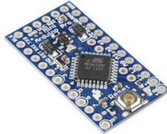
Figura 16: Arduino Pro Mini
