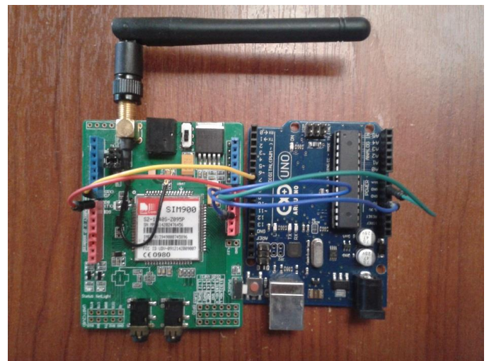
Fig. 4. ARDUINO MODULE connection with GSM / GPRS SIM900 - UART
