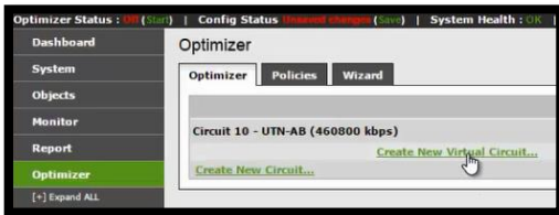
Figure 8. Creating a new virtual circuit. Extracted from EXINDA 4061 UTN.
