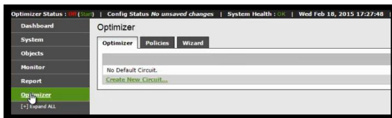
Figure 6. Creation of the new circuit. Extracted from EXINDA 4061 UTN.
