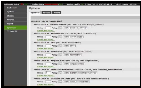
Figure 12. List of virtual circuits created. Extracted from EXINDA 4061 UTN.
