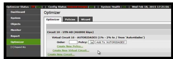
Figure 10. Viewing the new virtual circuit created. Extracted from EXINDA 4061 UTN.
