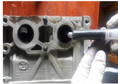
Fig. 4 Calculation of the volume of the standard exhaust duct.
