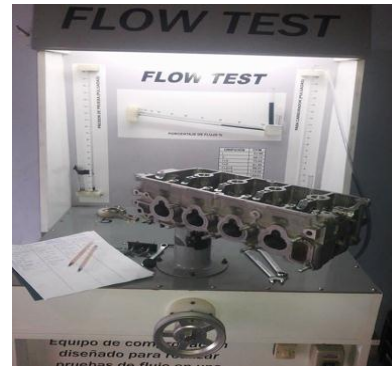
Fig. 9 Standard cylinder head test.
