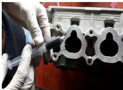
Fig. 3 Calculation of the volume of the standard intake duct.
