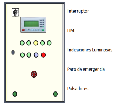
Fig 11 Control Panel Front Panel
