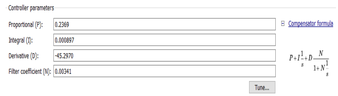
Fig 8 Characteristics of the transfer function applied a PID control
