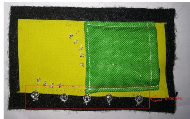
Fig. 46. Brooches for connection of sensors and GND in the detachable segment Source: Prepared by the author
