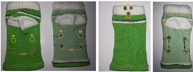
Fig. 52. Brooches connection to the harness and sensors Source: Prepared by the author
