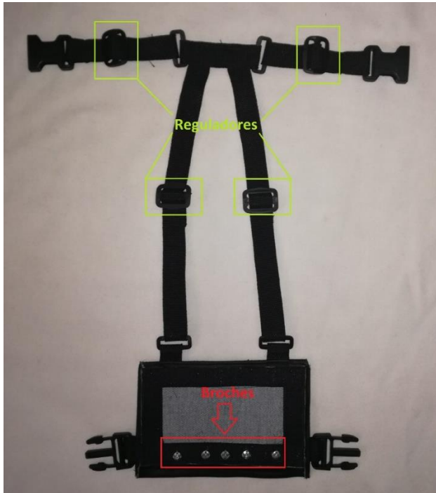
Fig. 48. Harness design and location of connecting brooches Source: Prepared by the author
