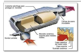
Of all emissions after combustion inside the engine, three gases emitted to be treated for their high toxicity, these are: carbon monoxide (CO), nitrogen oxides (NOx) and hydrocarbons (HC) to make this possible gas reaching the catalyst must reach a temperature of  $500\,^{\circ}$  C.
