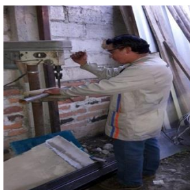
Figure 24: Drilling of various parts of the chassis. Source: Authors
