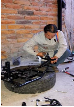
Figure 27: Assembling the direction of the chassis Source: Authors
