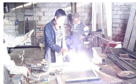
Figure 26: Union of chassis parts by MIG Source: Authors
