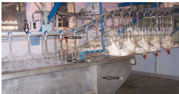
Figure 5.- Scalding chickens for production line immersion. Source: (Poultry Dressing plant Scalding or Chicken Scalding, 2013)
