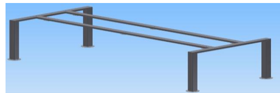
Figure 36: Design of the machine structure blanching chickens.
