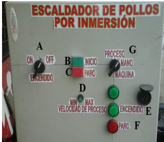
Figure 43: External elements for machine control.
