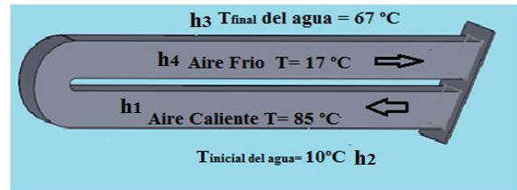
Figure 35.- Enthalpies in the heat exchanger transfer the bath water blanching.
