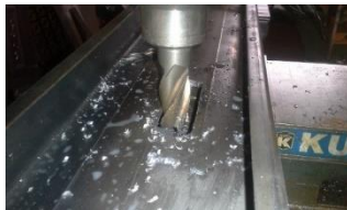
Figure 1: Drilling to adjust the band
