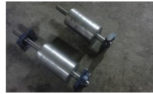
Figure 3: Check roller shafts for bearings
