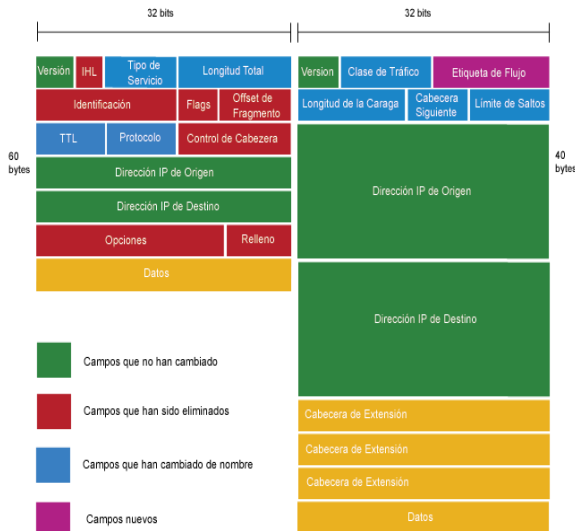
Fig. 1 Format of the head-board IPv6
