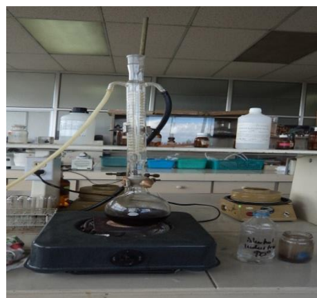
Photo: Equipment reflux.
