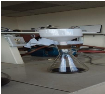
Photo: Filtration with drain pump.
