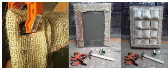
Fig. 15. Immobilization of the substrate in the panel and stapling
