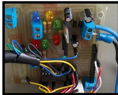
**Figura 2. 14** Circuito conversor 5-10 VDC
