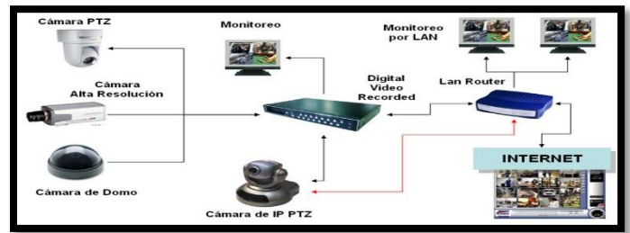
Figure 1. Basic outline of an IP video surveillance system.
