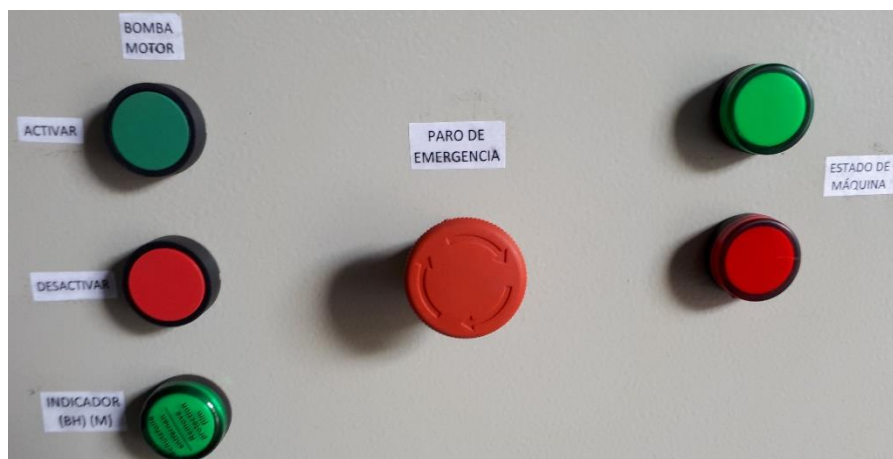
Figura 36: Panel frontal del tablero
