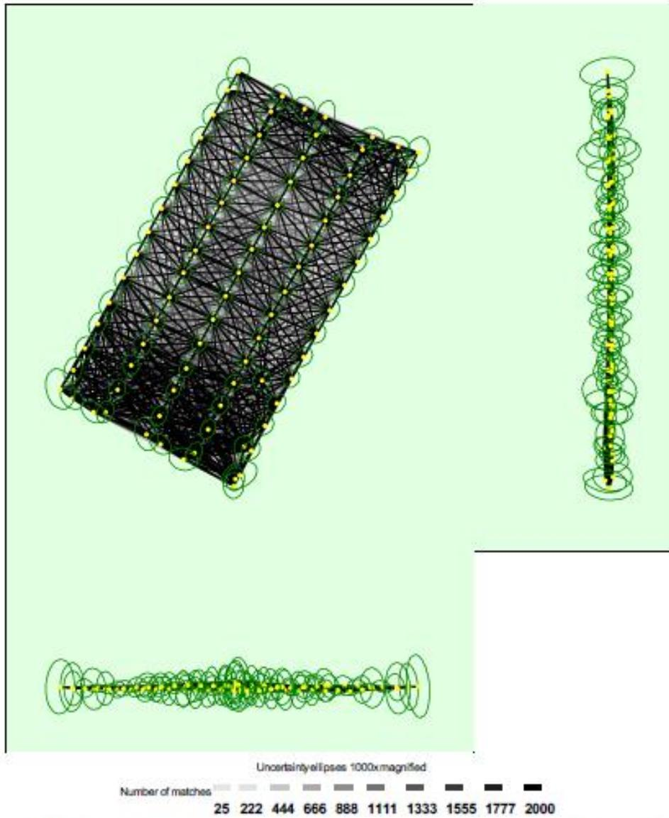
Figure 2: Computed image positions with links between matched images. The darkness of the links indicates the number of matched 2D keypoints between the images. Bright links indicate weak links and require manual fix points or more images. Dark green ellipses indicate the relative camera position uncertainty of the bundle block adjustment result.
