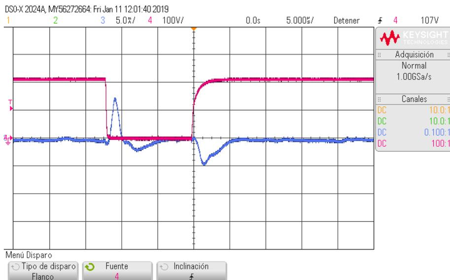
**Figura 55. Ch 3 escala 5.0mA, Ch 4 escala 100V, Level 106.525V, escala principal 5.000us**
