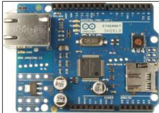
Fig. 1.15 Escudo Arduino Ethernet.
