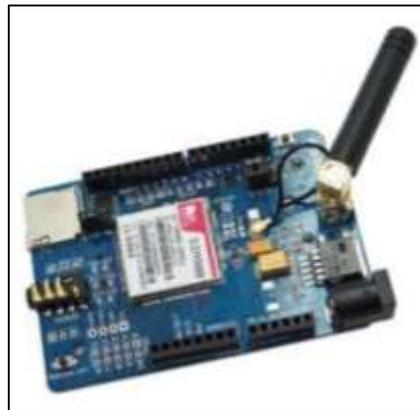
Fig. 2.3 Shield GSM GRPS SIM900.
