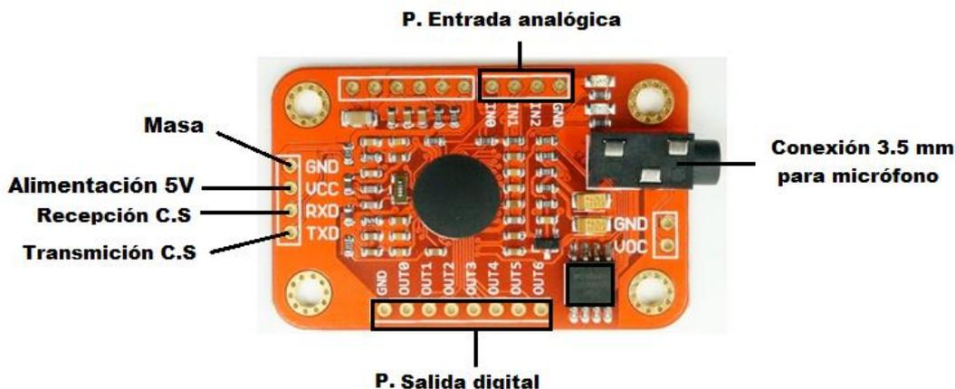
**Figura 1.23** Microcontrolador Elechouse V3
