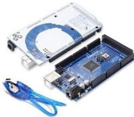
**Figura 1.15** Arduino Mega 2560
