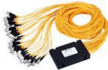
SPL1101 series products directly lead out 3m pigtailed mainly installed in a tray to implement splitting and cable distribution functions. The splitting ratio covers 1:2~1:64 even splitting and 1:2 (5/95, 10/90, 30/70) uneven splitting.
