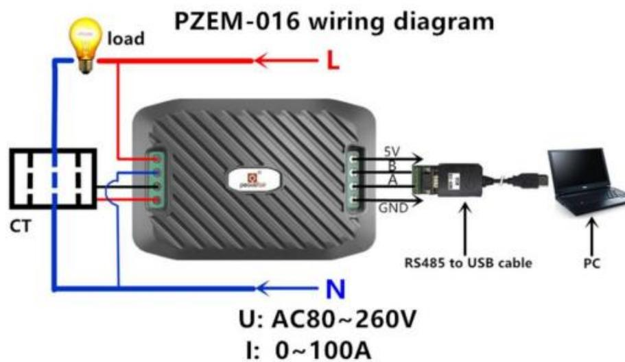
Picture 4.2 PZEM-016 wiring diagram
