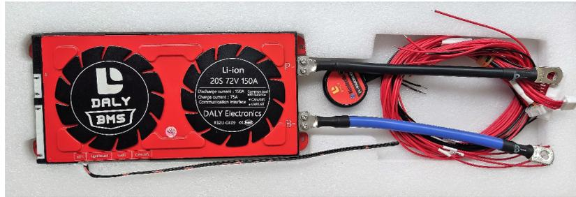
Figura 4.18: BMS Daly modelo Smart li-ion 72V 20s 150A
