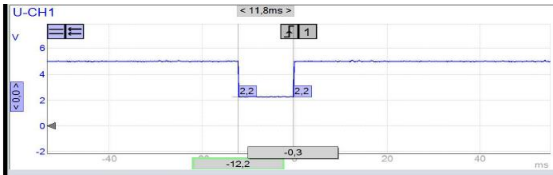
Figura 3.24 Oscilograma sensor CMP falla 3
