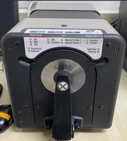
A black and silver X-Rite Color i 5 spectrophotometer. The front panel features a control panel with various settings and a large circular lens. The lens has a '60MM' label. The control panel includes sections for 'Aperture', 'UV', and 'Specular', each with several checkboxes and labels like '065', 'Adjusted Position 1', 'Included', 'Excluded', 'Adjusted Position 2', 'Excluded', 'Transmission', 'Reflection', 'NoPuffler 65', and 'Calibrated 65'. |
