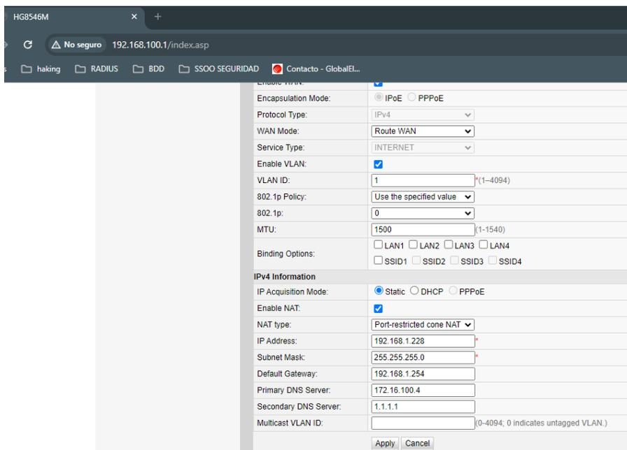
The screenshot shows the configuration page for a HG8546M router. The browser address bar indicates the URL is 192.168.100.1/index.asp. The configuration is for a WAN interface. Key settings include:
