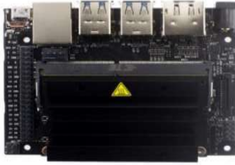
Fig. 2.27 Placa microcontrolada NVIDIA Jetson Nano [33]
