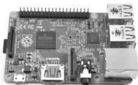
Fig. 2.25 Placa microcontrolada Raspberry Pi [31]
