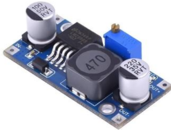
Figura 4.7: Conversor DC-DC Step-Down LM2596
