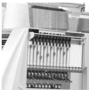
c. - The needle bed holds the needles, in this type of machine has other elements in each slot or channel that help to form stitches, retained, tuck, stitches transfer, etc. And these are also of the needle (A), the heel of the needle (B) or coupling piece (needles of these machines have no heel), the intermediate pretty flat (C), and selector (D).
