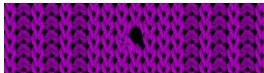
There you can see clearly in the center of the drawing that the mesh where the draft has the inclination to the left and joins the back of the fabric.
