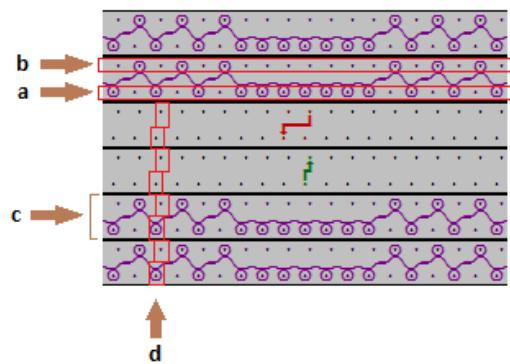
At first sight, it can be appreciated that the way needles are represented is different. In this case, there are no vertical lines but there are points, each point represents a machine needle.
