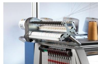
At the bottom of the friction feeder system, it has another thread side recuperators system which is the thread control unit used to recover the thread at the time the carriage changes direction to always keep it
