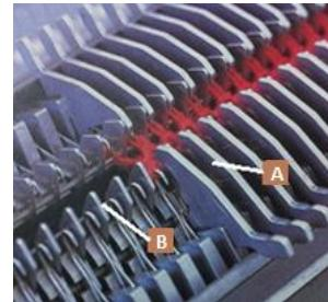
h. - The needle bed of the machine is controlled by an engine that allows making big moves up to 4 inches and a programmable speed to perform a wide range of designs. In the picture you can see that the back needle bed is moved to the left with respect to the front needle bed.
