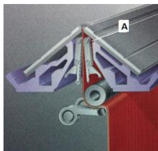
j. - The yarn feeders do not differ greatly from those of manual machine in form and the goal is to guide the yarn directly to the needles at the right time in need. The machine has 8 yarn feeders on each side, 16 in total and has a strand of yarn on either side and
