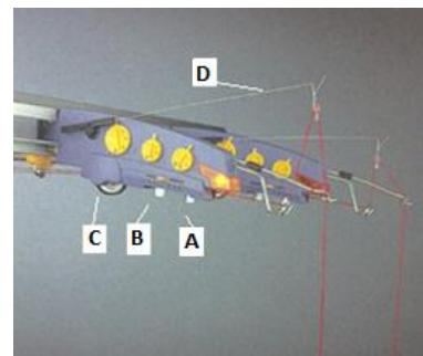
b. - The yarn coming from the cone travels from the creel by means of the thread detector and feeds through friction when a little hard materials need a little more help to pull the yarn, this is done by means of two ceramic rollers are constantly turning.
