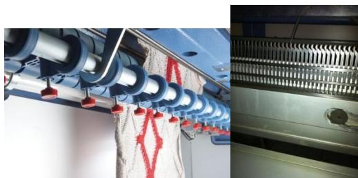
Besides the fabric take down the machine has an auxiliary take-down (A) that is located on the fabric take-down and immediately under the needle bed and can be turned on or off depending on the need, this helps especially when the machine make widening and narrowing.
