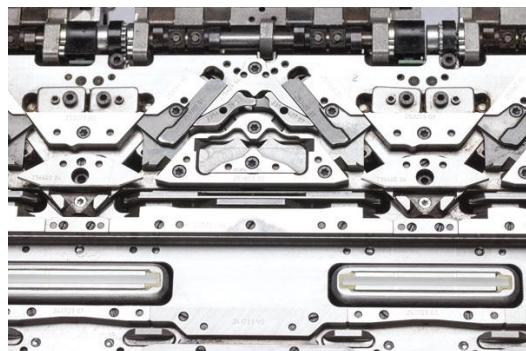
In the upper weaving system are brushes, one for the front needle bed and another to the back, which helps to maintain constantly open tabs needles so they can make the yarn supplied by the yarn feeder.
