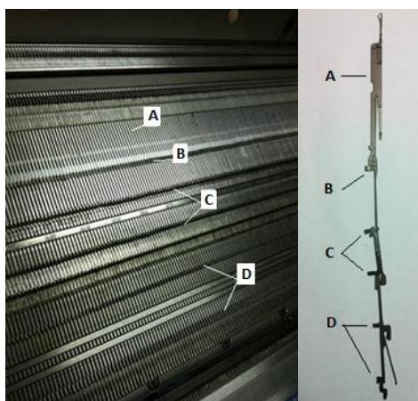
d. - The system contains knitting cams and bolts, some of them other are fixed and others are mobile. They are traveling road in which the heels of the needles form stitches, transfer, etc. All these elements are located on a metal plate which is attached to the carriage.
