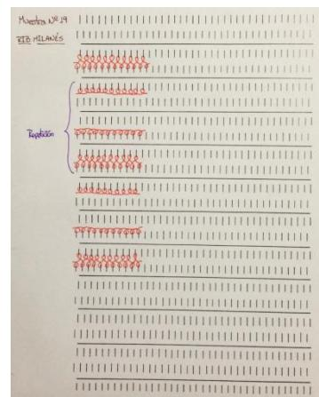
At the time of technical schemes using a pointer or a pin to go guided tissue with each pass and go noting whether it is being woven mesh front, mesh back, floating or tuck stitches. In times
