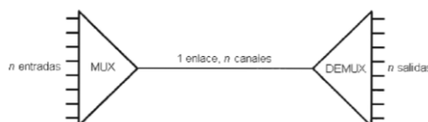
Figure 2 Basic multiplexing scheme Source: (Cisco Systems, Inc., 2001)
