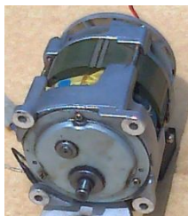
Figure 12. External appearance AC gearmotor
