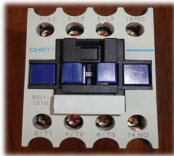
**FIGURA 60:** Contactor NC1-12
