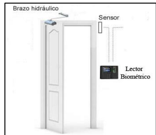
Figure 12. System Access Control Data Center. Source: http://st-ingenieria.com/corrientes-debiles/control-de-acceso/
