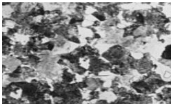
Figura 44. 25-mm (1-in.) diam 4140 steel bar, austenitized 1 h at 845 °C (1550 °F), cooled to 650 °C (1200 °F)
