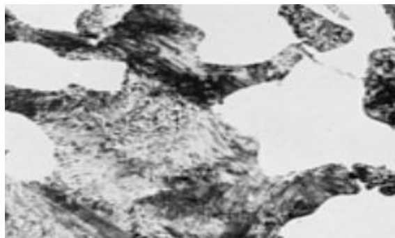
Figura 47. 4130 hot-rolled steel bar, 25 mm (1 in.) in diameter, annealed by austenitizing at 845 °C (1550 °F)
