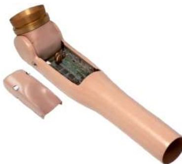
Figura 1.3 Brazo Digital Boston (Liberating Technologies, Inc., 2017)
