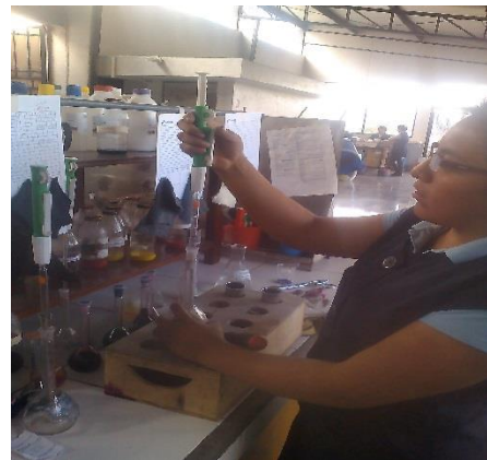
Figure. 1. Dosage of dyes performed manually. (Indutexma, 2016)
