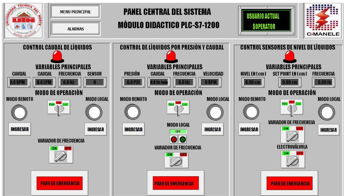
Fig. 6.20 HMI PLC S7-1200
