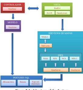
Figure 3 Architecture of the System Source: Owner
