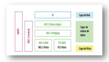
Figure 3 PLC Protocol Stack [5]
