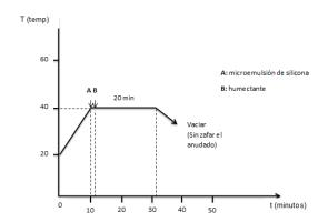
**Results:** In this test it was observed that the finishes of ruching are formed properly, but it does not have resistance to ironing since the percentage of silicone microemulsion is minimal.
