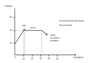
**Results:** In this process it was observed that the ruching resist washing tests, rubbing and ironing, so these show similar characteristics to the previous test, but if it increases the silicone, the microemulsion becomes a more viscous bath which lowers the level of exhaustion.
