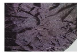
**Ironing:** Resists temperatures as low as  $55 \,^{\circ}$  C, if the temperature is increased, the ruching disappears rapidly  $(78 \,^{\circ}$  C).
