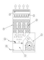
Figures 16. Parts of a cooling tower.
