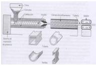
Figure 3. Equipment for extrusion profiles.
