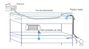
Figure 12 Cooling System Water recirculation.
