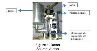
When the operator needs to stop the dispensing machine lifting lever stop doing raise swivel shaft cam, so the yogurt leaves descend. For the placement of the yogurt into the hopper the operator should position the product with the help of a ladder.
