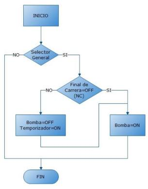
Figure 18. Flowchart of the level Control
