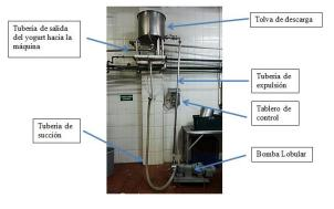
Figure 19. Assembly of the elements of the level Control System Source: Author
