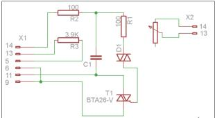
Figure 11. Horizontal sealing Power Board Source: Author
