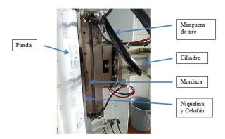
Figure 5. Elements of sealing vertical Source: Author
