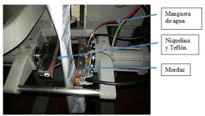
Figure 6. The Horizontal sealing elements Source: Author
