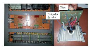
Figure 12. Horizontal sealing Power Board Source: Author
