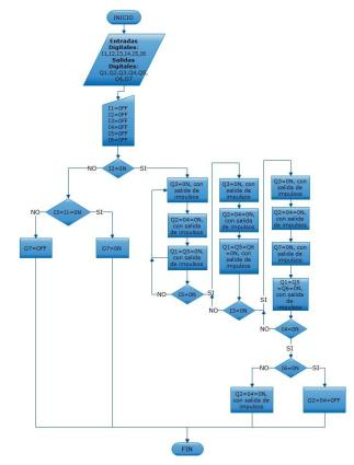
Figure 17. Flowchart of the automatic system of the machine Source: Author
