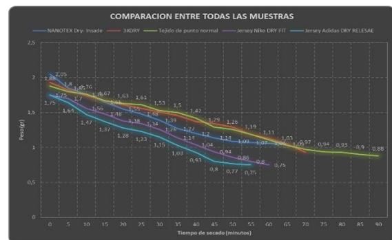
Weight ratio of absorption time between all samples compared
